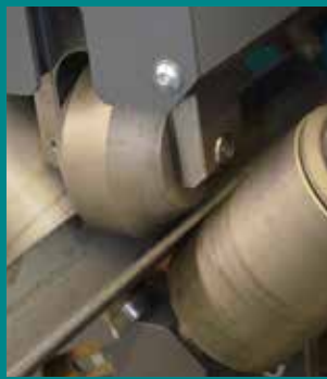
Automatic measurement of the material thickness
