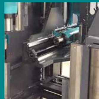
Solid spindle guide ideal for lateral milling force.
