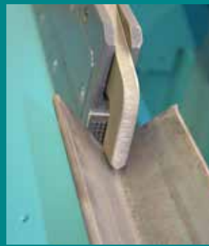
Universal gripper for processing angle and flat steel
