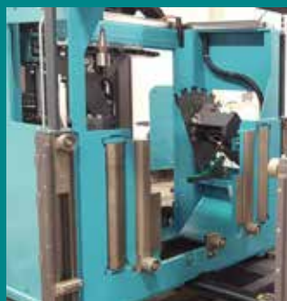
Robust clamping system and large tool changer.
