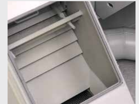
Multi-level cascade air cleaner for ideal separation of dust and mill scale from abrasive to achieve dust free, reusable abrasive for optimal cleaning effect and minimal wear to the machine.
