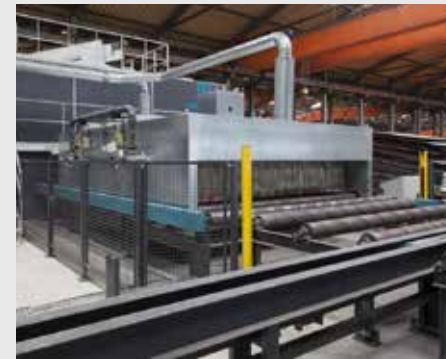
Energy saving and fully isolated Pre-heaters ensures the right material temperature before painting.
