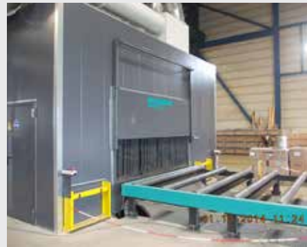
An additional slide at the inlet and outlet side of the machine enables processing of variable material heights.
