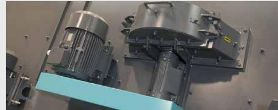
Easy accessible heavy duty indirect v-belt driven twin disc turbines with 8 blades. KALTENBACH uses a sub-frame for the assembly of the turbines for even better stability of the machine, thereby reducing oscillations and noise hindrance. The KALTENBACH high capacity turbines are statically and dynamically balanced.
