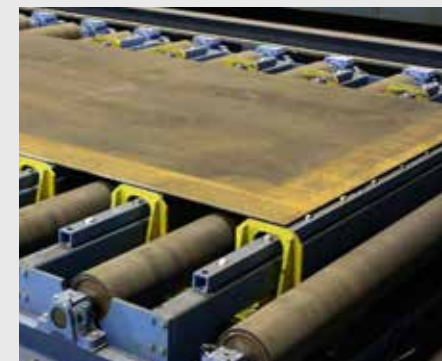
Within the roller conveyor integrated automatic alignment system for plates for quick and easy loading by overhead crane.
