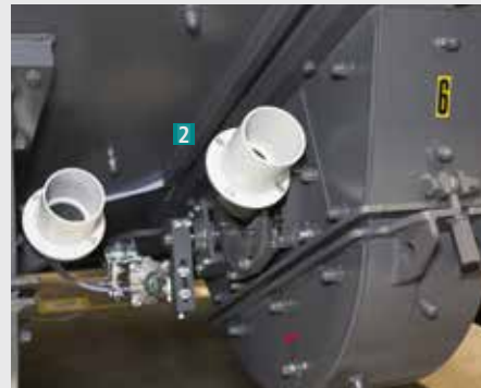
The blast pattern of the turbines is automatically adjusted to the material offered to the machine to avoid ineffective blasting and additional wear to the machine.
