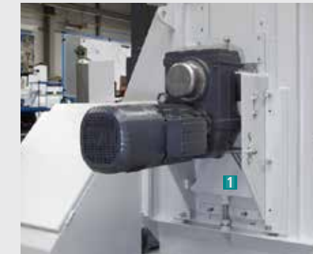
Elevator equipped with easily adjustable sub frame for tensioning of the elevator belt. Due to the subframe the elevator tensioning is a one man job by adjusting only one bolt (1).
