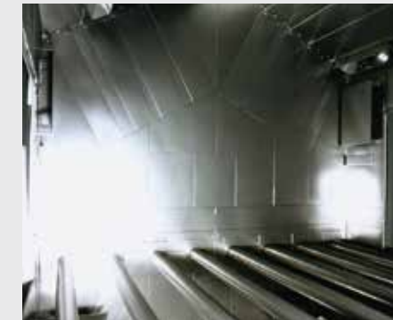
Manganese lining covered walls and short roller distance allows transport of material lengths starting from 2500 mm upwards.
