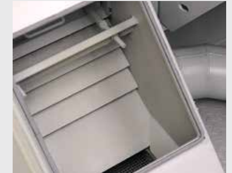
Multi-level cascading air cleaner for ideal separation of dust and mill scale from abrasive to achieve dust free, reusable abrasive for optimal cleaning effect and minimal wear to the machine.
