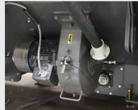
Direct driven twin disc turbines with 8 blades.
