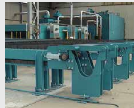
Integrated automatic bundle system for ready blasted and painted material for easy packing.
