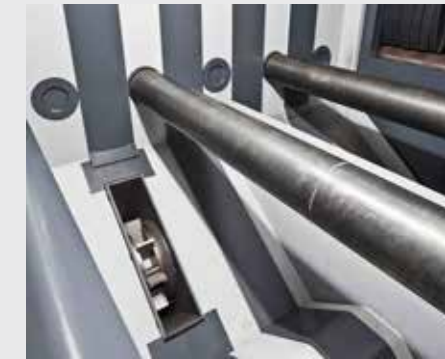
Solid hardened transport rolls inside the blaster. Turbines positioned not in line with each other to avoid individual interference.
