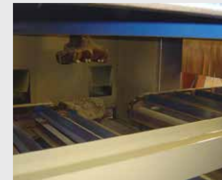
Reduced overspray through precise contour determination of the surfaces to be coated and exact control of spray guns.
