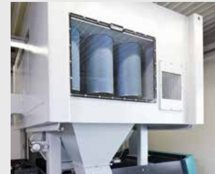
Optimal air filtration by latest generation highly effective exhaust plant.
