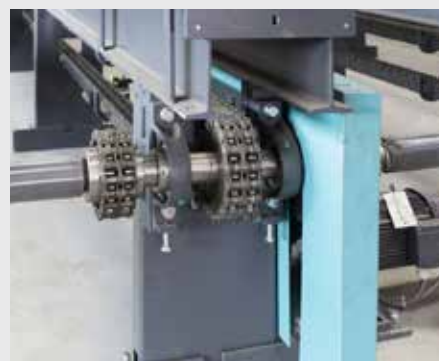
Heavy duty double chain drive for more stability.
