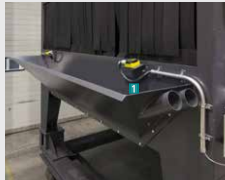
Machines with entrance dimensions starting from 2500 mm upwards are standard equipped with measuring systems of the material width (1), in combination with adjustable turbines (2).
