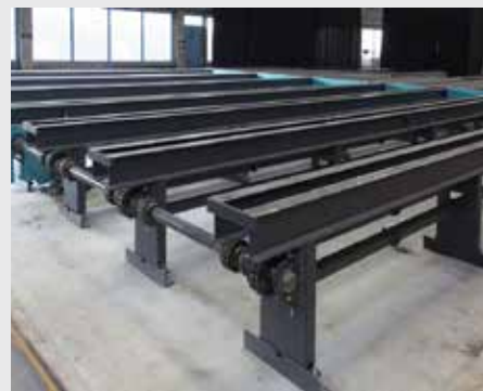
Cross transport beams for easy loading and unloading up to 20 m single lengths. Lift and Go system equipped with lifting trolley and power packs per stillage and a lifting height of 120 mm.
