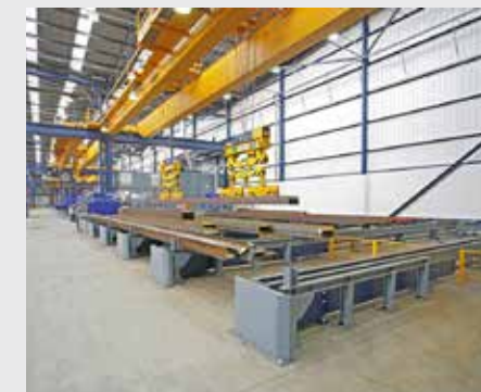
Special protection plates at the end of the cross stillages to prevent damage by lorries and side loaders.
