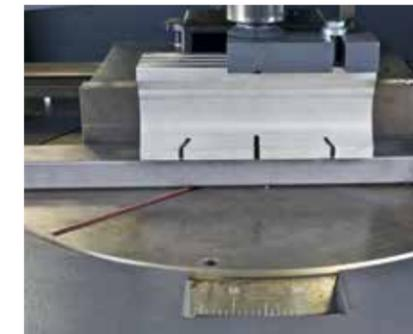
CNC-controlled cutting angle setting.
