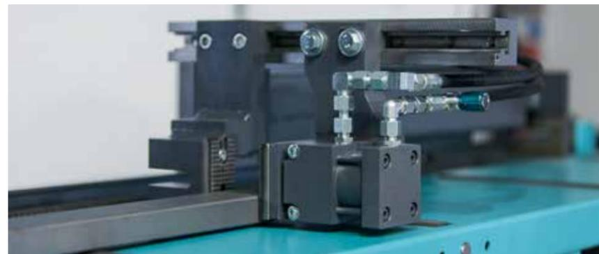
Infeed measuring device M 45 NC for the automatic material feed (KKS 400H/KKS 450 H). Alternatively used as a NC-controlled length stop. The M 45 NC clamps the material at the bar end and is driven forward automatically according to the programmed length.
