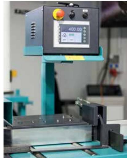
Length measurement device L 41 NC
