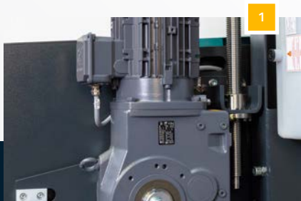
Electronic feed control by ball screw spindle
