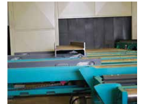
Cross-conveyor with lifting carriage especially for profile bundles, layers and plates.
