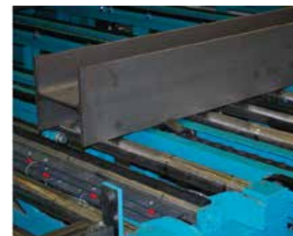
Cross-conveyor with drag chains for robust and low-maintenance transport.
